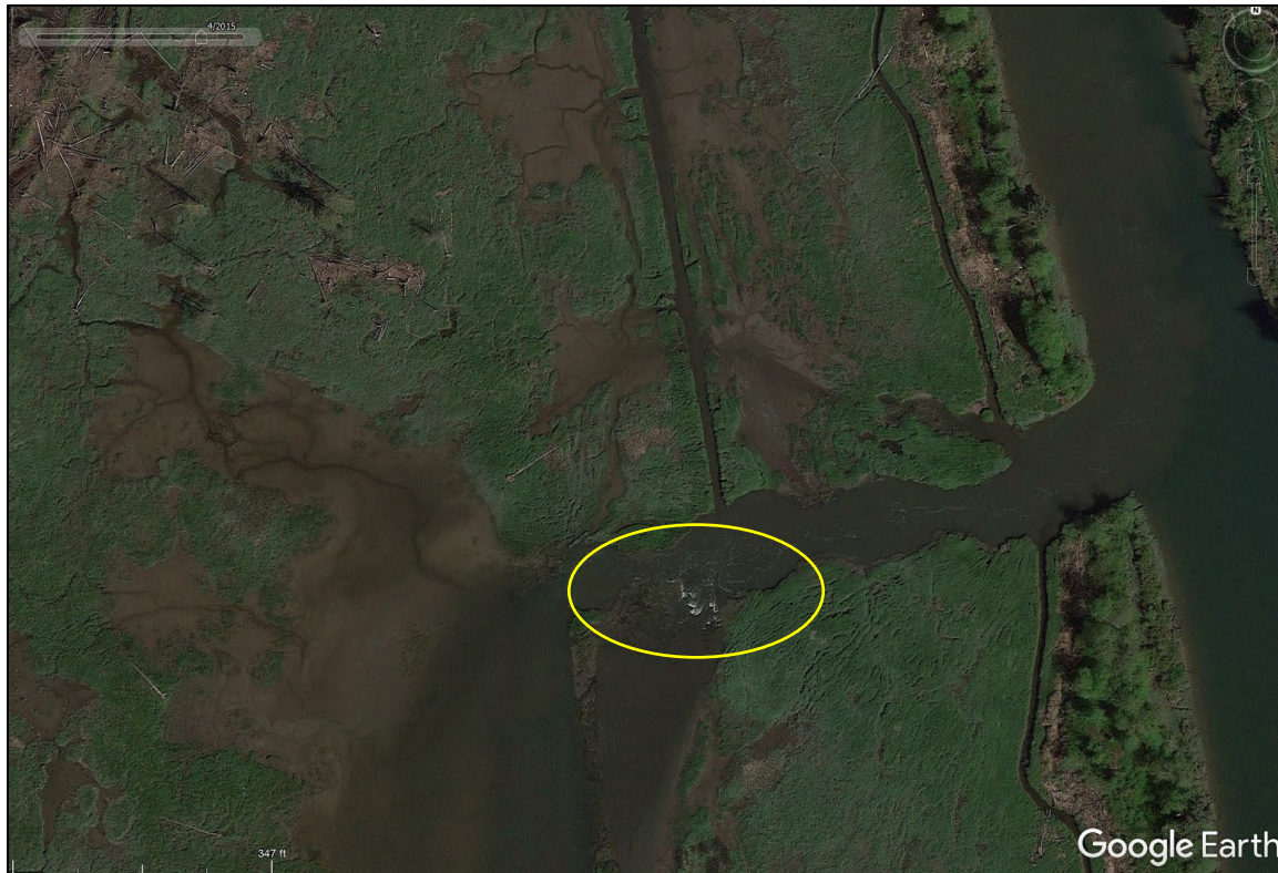
Figure 22. Low tide erosion of marsh plain into main breach channel due to undersized ditch showing formation of velocity barrier (hydraulic jump)
